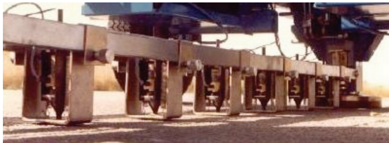
Figure A.2: Deflection sensors of the geophone type (source COST 336)
