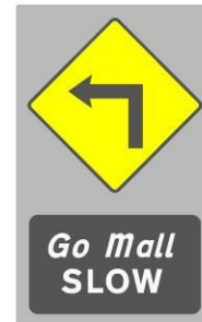
Figure 3.14: Vehicle Activated Sign for Sharp Bend (Sign W 050L with SLOW)
