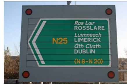
Figure 3.1: Typical Rotating Prism VMS
