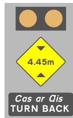
Figure 3.15: Vehicle Activated Sign for Low Bridge (Sign W 110 with Signals S 102 and TURN BACK)
