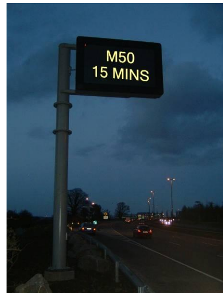
Figure 3.6: Single Colour Full Matrix VMS
