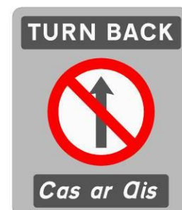
Figure 3.16: Sign F 903, Turn Back, as Vehicle Activated Sign
