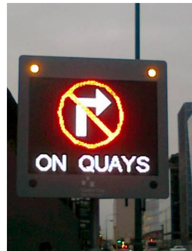
Figure 3.7: Dual Colour Full Matrix VMS
