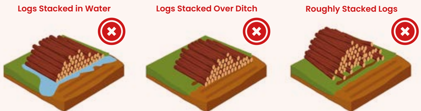
Figure 2: Advice for stacking timber in the forest.
