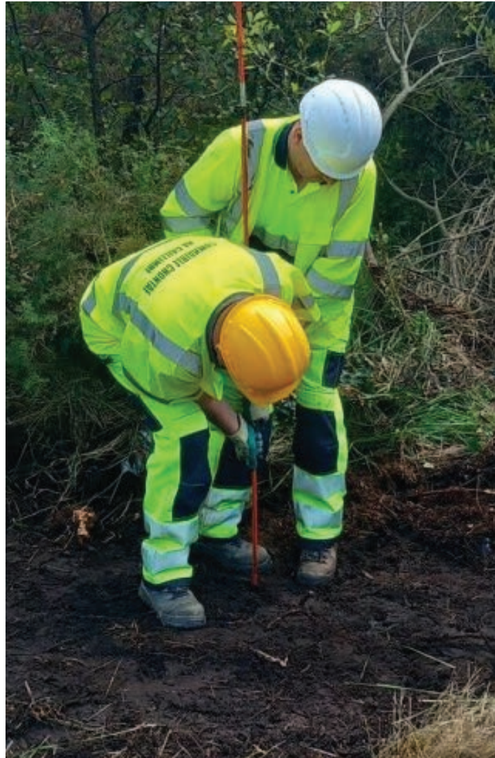
Figure D.1.1 – Photograph Showing Manual Peat Depth Probing.
