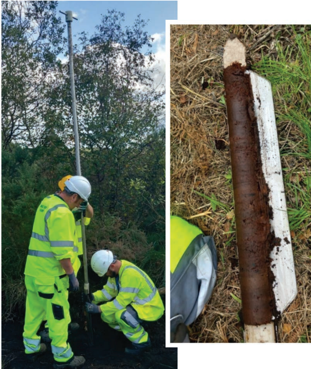
Figure D.1.2 – Photographs Showing Russian Peat Core Sampler.
