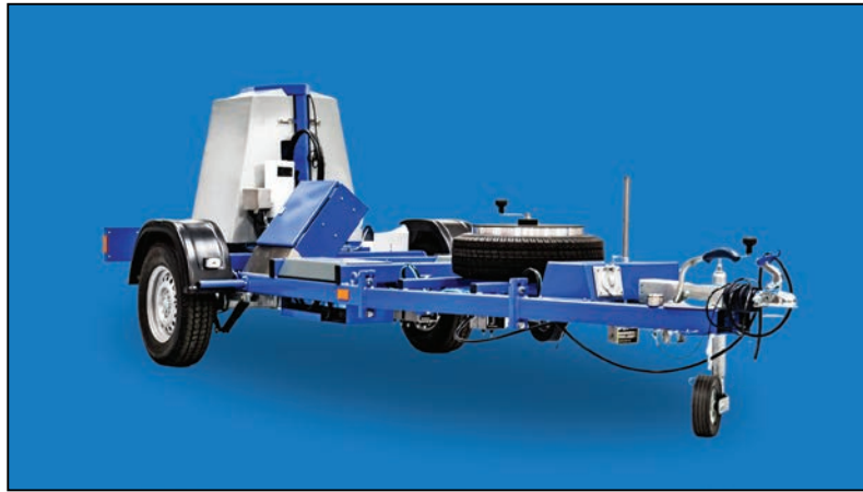
Figure 3.3 - Falling Weight Deflectometer Testing Device
