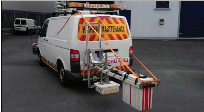
Figure 3.4 - Ground Penetrating Radar
